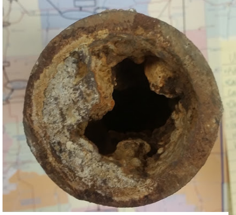
Figure 4-7 Calcium Carbonate Precipitate
