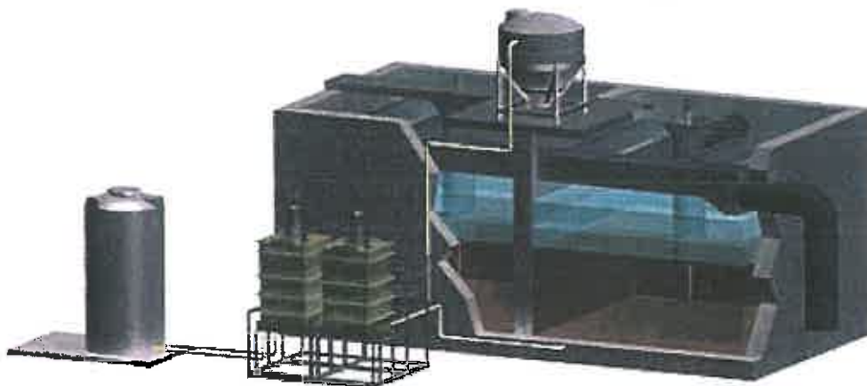
Figure 4-6 MIEX Treatment System: High Rate Configuration
